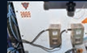
left : odor sensor unit right : photocatalyst device ©NASA/Axiom Space
