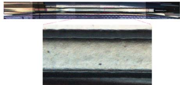
Cellulose enzymatically synthesized in microgravity is uniformly synthesized
